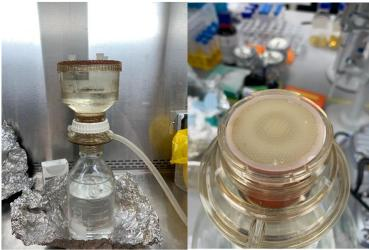
Microorganisms in water such as bacteria are collected by passing water through filters, which function as sieves. Scientists then extract and study the genetic material of the microorganisms trapped on the filters.
