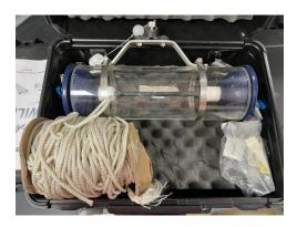
Water from quarry lakes is collected using a water sampler designed for collecting water from water bodies such as lakes.
