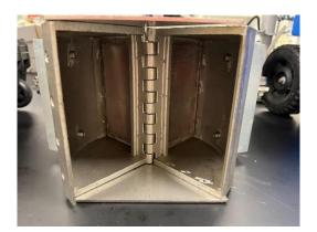
Sediment from the bottom of quarry lakes is collected using a sediment grab. It has two jaws which close and grab sediment when it is lowered to the lake bottom.
